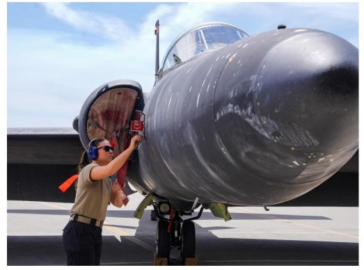
U.S. Air Force Airman Josephine Killey, 9th Aircraft Maintenance Squadron crew chief apprentice, replaces the red pins on a U-2 Dragon Lady during its recovery at Beale Air Force Base, California, June 18, 2024. Replacing the pins during recovery is a crucial step to prevent accidental activation of systems while maintainers work on or around the aircraft. (U.S. Air Force photo by Staff Sgt. Shaei Rodriguez)
