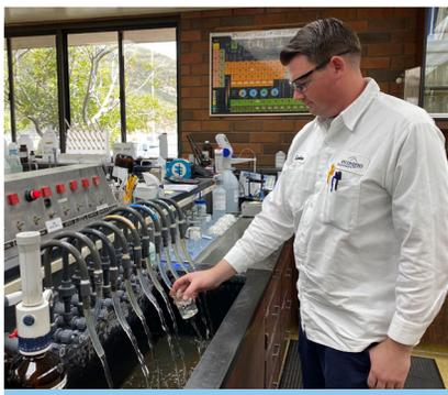
At the Water Treatment Plant (WTP), water samples are collected continuously by the Plant Operations staff during various stages of the treatment process. Testing is performed on alkalinity and turbidity in the raw water source; during the period that the water is being treated, monitoring takes place for coagulation, settling, and for fluoride and chlorine levels. Constant adjustments are made to the treatment process based upon the results from sampling and testing performed at the WTP.
