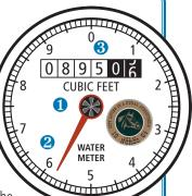
Weter Register — The meter register is a lot like the odometer on your car. The numbers keep a running total of all the water that has passed through the meter. The register shown here indicates that 89,505 cubic feet of water has passed through this
