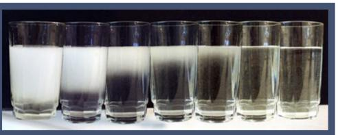
the rapid reduction in pressure causes the air to come out of solution, and creates the milky look you see. If this is the case, it will clear before your eyes as in the picture.
