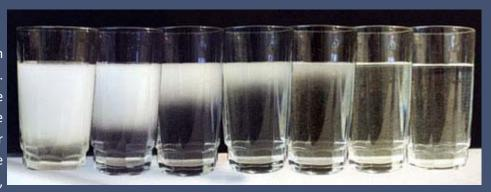
the rapid reduction in pressure causes the air to come out of solution, and creates the milky look you see. If this is the case, it will clear before your eyes as in the picture.
