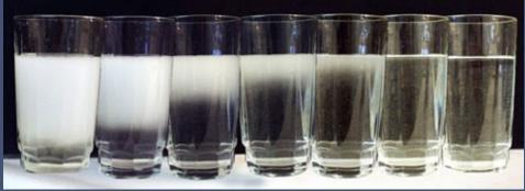
potential to release that air. When you turn on your tap, the rapid reduction in pressure causes the air to come out of solution, and creates the milky look you see. If this is the case, it will clear before your eyes as in the picture.
