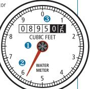
Other Register — The meter register is a lot like the odometer on your car. The numbers keep a running total of all the water that has passed through the meter. The register shown here indicates that 89,505 cubic feet of water has passed through this meter.
