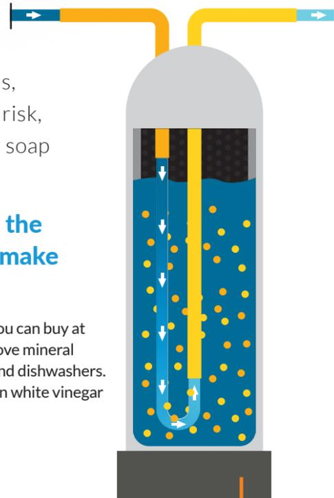
A water softener works by using a process called ion exchange to remove calcium and magnesium ions from hard water.
