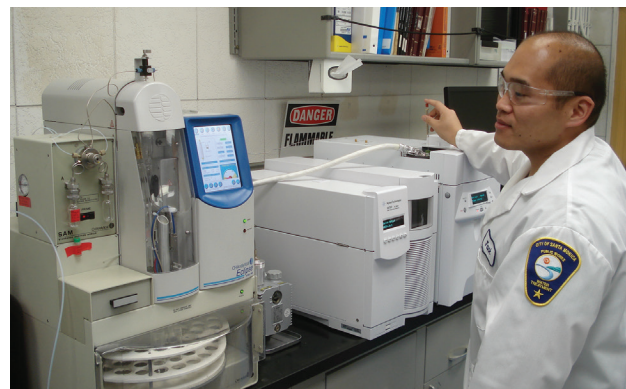
Using gas chromatography mass spectrometry (GC/MS), chemists test for volatile organics in the water.
