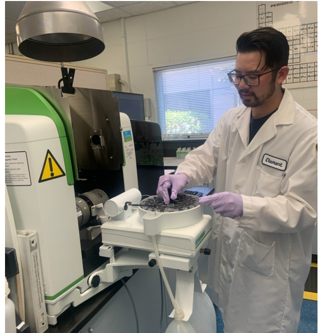
Using atomic absorption spectrometry (AAS) technology, chemists routinely monitor the water quality of the City's drinking water.
