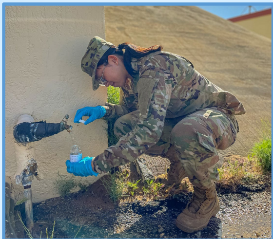
Pictured above: A technician from the 412th Operational Medical Readiness Squadron, Bioenvironmental Engineering Flight, conducting routine water testing at locations spanning the water distribution system. Water samples are collected, tested by a certified laboratory, and results are submitted to the State Water Resources Control Board to demonstrate compliance with all requirements and regulations.
