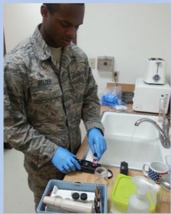
Pictured above: Technicians from the 412th Operational Medical Readiness Squadron, Bioenvironmental Engineering Flight conducting routine water testing at locations spanning the water distribution system. Water samples are collected, tested by a certified laboratory, and results are submitted to the State Water Resources Control Board to demonstrate compliance with all requirements and regulations.
