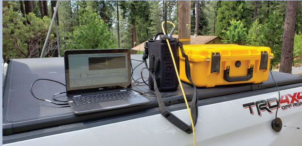
Leak Detection Equipment used to help pinpoint location of leak
