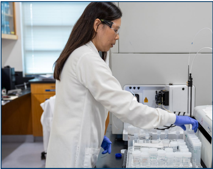
A DSRSD employee sets up an autosampler to test drinking water for lead and copper concentrations.
